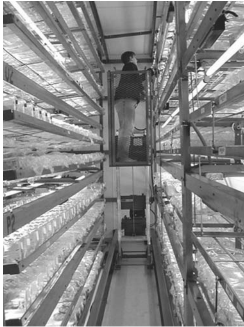
Figure 4. Floor to ceiling arrangement of open-frame shelving in 3.7 m culture room.
