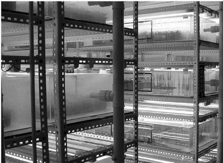
Figure 2. A photoautotrophic micropropagation system using large vessels with forced ventilation, installed for commercialization in Kunming, Yunnan Province, China.
