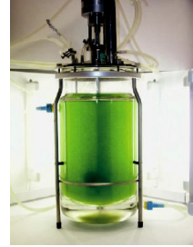
Fig. 3.8 Greenovation use a fully contained moss bioreactor. This company has established an innovative production system for human proteins. The system produces pharmacologically active proteins in a bioreactor, utilizing a moss ( Physcomitrella patens ) cell culture system with unique properties [24].
