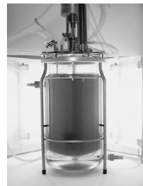
Fig. 8 Greenovation use a fully contained moss bioreactor. This company has established an innovative production system for human proteins. The system produces pharmacologically active proteins in a bioreactor, utilizing a moss ( Physcomitrella patens ) cell culture system with unique properties [24]. (See Color Plate p. xxi).
