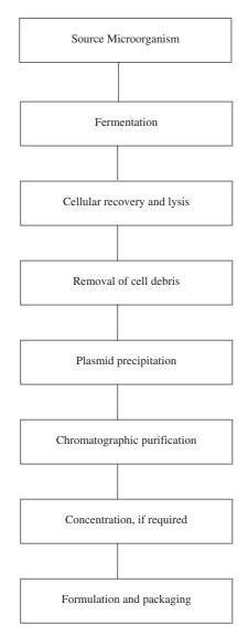
**Figure 14.11** Overview of the manufacturing process for the large-scale production of plasmid DNA. Refer to the text for further details
