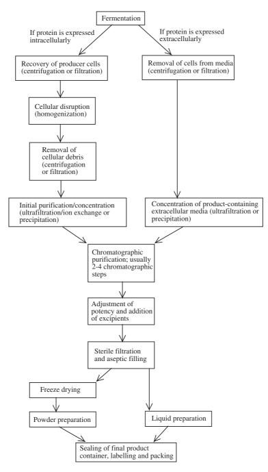
**Figure 6.1** Overview of a generalized downstream processing procedure employed to produce a finishedproduct (protein) biopharmaceutical. QC also plays a prominent role in downstream processing. Qualty control personnel collect product samples during/after each stage of processing. These samples are analysed to ensure that various in-process specifications are met. In this way, the production process is tightly controlled at each stage
