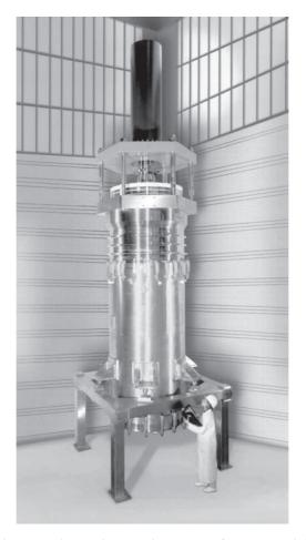
Figure 11.4 Process-scale HPLC column. Photograph courtesy of NovaSep Ltd, http://www.novasep.com
