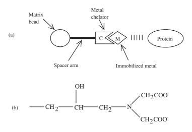
**Figure 6.17** Schematic representation of the basic principles of metal chelate affinity chromatography. Certain proteins are retained on the column via the formation of coordinate bonds with the immobilized metal ion (a). The actual structure of the most commonly used metal chelator, iminodiacetic acid, is presented in (b)
