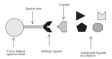
**Figure 6.14** Schematic representation of the principle of biospecific affinity chromatography. The chosen affinity ligand is chemically attached to the support matrix (agarose bead) via a suitable spacer arm. Only those ligands in solution that exhibit biospecific affinity for the immobilized species will be retained
