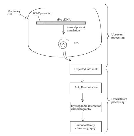
**Figure 5.2** The production and purification of tPA from the milk of transgenic goats. (WAP promoter: murine whey acid promoter). The downstream processing procedure yielded in excess of an 8000-fold purification factor with an overall product yield of 25 per cent. The product was greater than 98 per cent pure, as judged by sodium dodecyl sulfate (SDS) electrophoresis
