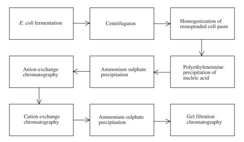
**Figure 11.9** Production of rhGH in *E. coli* (as an intracellular protein). Subsequent to fermentation, the cells are collected by centrifugation or filtration. After homogenization, nucleic acids and some membrane constituents are precipitated by the addition of polyethyleneimine. Ammonium sulfate precipitation of the supernatant concentrates the crude rhGH preparation. Chromatographic purification follows, as illustrated
