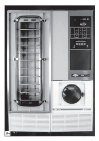
**Figure 6.25** Photographic representation of (a) laboratory-scale, (b) pilot-scale and (c) industrial-scale freeze-driers. Refer to text for details. Photograph courtesy of Virtis, USA
