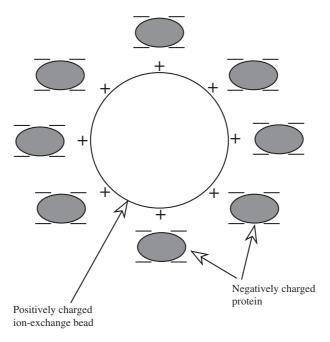
**Figure 6.11** Principle of ion-exchange chromatography, in this case anion exchange chromatography. The chromatographic beads exhibit an overall positive charge. Proteins displaying a nett negative charge at the pH selected for the chromatography will bind to the beads due to electrostatic interactions
