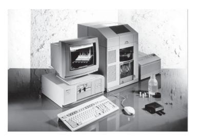
**Figure 7.2** Photograph of a capillary electrophoresis system (the HP-3D capillary electrophoresis system manufactured by Hewlett Packard). Refer to text for details. Photograph courtesy of Hewlett Packard GmbH, Germany
