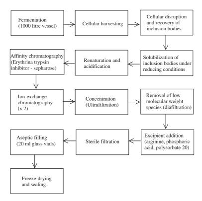
**Figure 12.12** Production of Ecokinase, a modified tPA molecule that gained regulatory approval in Europe in 1996. The production cell line is recombinant *E. coli* K12, which harbours a nucleotide sequence coding for the shortened tPA molecule. The product accumulates intracellularly in the form of inclusion bodies
