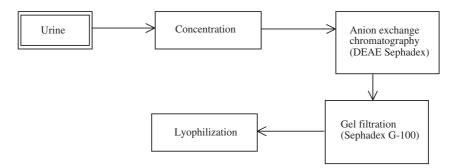
**Figure 11.11** Overview of the procedure by which hCG may be purified from the urine of pregnant females at laboratory scale. Production-scale systems would be at least partially based upon such a purification strategy. Although initial concentration steps could involve precipitation, the use of ultrafiltration would now be more common
