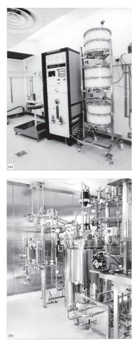
**Figure 13.11** Photographs illustrating some cleanroom-based processing equipment utilized in the manufacture of SmithKline Beecham's hepatitis B surface antigen product. (a) A chromatographic fractionation system, consisting of (from left to right) fraction collector, control tower and chromatographic columns (stacked formation). (b) Some of the equipment used to formulate the vaccine finished product. Photograph courtesy of SmithKline Beecham Biologicals s.a., Belgium
