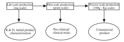
**Figure 4.9** Scale-up of proposed biopharmaceutical production process to generate clinical trial material, and eventually commercial product. No substantive changes should be introduced to the production protocol during scale-up
