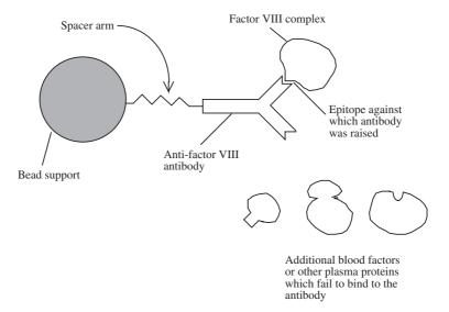
**Figure 12.7** Purification of factor VIII complex using immunoaffinity chromatography. The immobilized anti-factor VIII antibody is of mouse origin. Antibodies raised against specific epitopes on both the VIII:C and vWF components have both been successfully used. Industrial-scale columns would often exhibit a bed volume of several litres. Note that the different elements in this diagram are not drawn to the correct scale relative to each other
