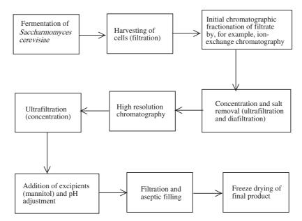
**Figure 12.9** Overview of the production of Refludan (recombinant hirudin). The exact details of many steps remain confidential for obvious commercial reasons. A number of QC checks are carried out on the final product to confirm the product's structure. These include amino acid composition, HPLC analysis and peptide mapping
