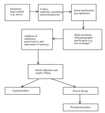
**Figure 13.1** Overview of the production of antisera for therapeutic use to induce passive immunization. Refer to text for specific details
